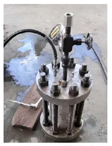
The FlexSleeve® joint was successfully hydrostatic tested to 365 bar (5,200 psi) after welding.
