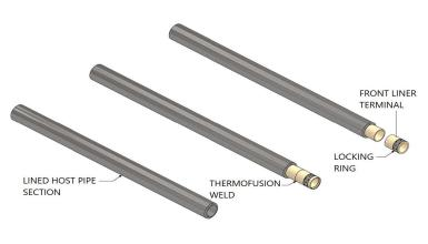
Step 4: Insert SealSleeve™ into pipe end, align pipe sections, and perform girth weld.
